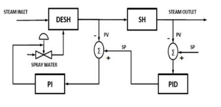
Figure 1: DESH based SH steam temperature control
